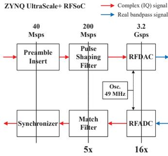
Fig. 4. RFSoc 4x2 digital-to-analog interface block diagram.
