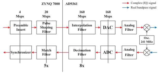
Fig. 3. ADRV9361-Z7035 digital-to-analog interface block diagram.
