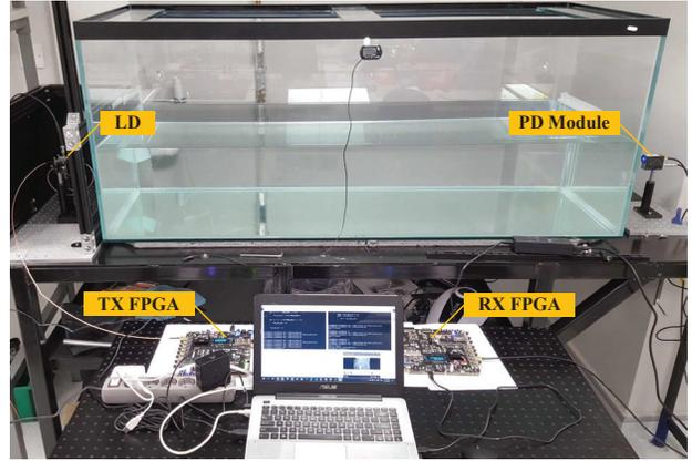
Fig. 6. Photograph of UOWC experiment setup with LD, PD, and a 1.5m water tank.
