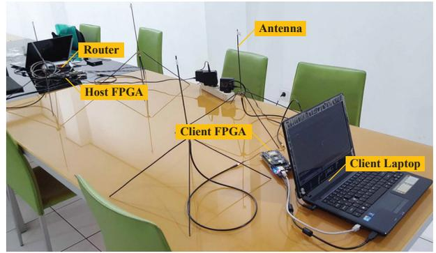
Fig. 5. Photograph of RF experiment setup with a 1/4 wave antenna at a distance of 1.5 m.
