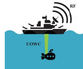
Fig. 1. An illustration of a hybrid RF-UOWC system. The above-water communication uses RF, while underwater communication uses UOWC.
