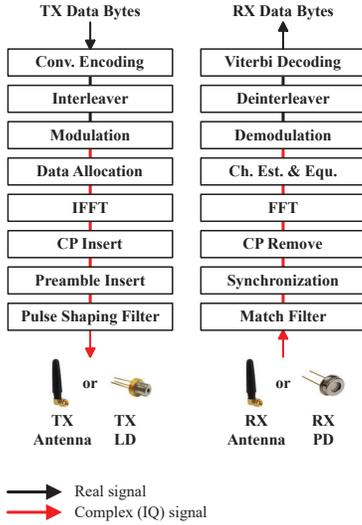
Fig. 2. Block diagram of the OFDM processor datapath.
