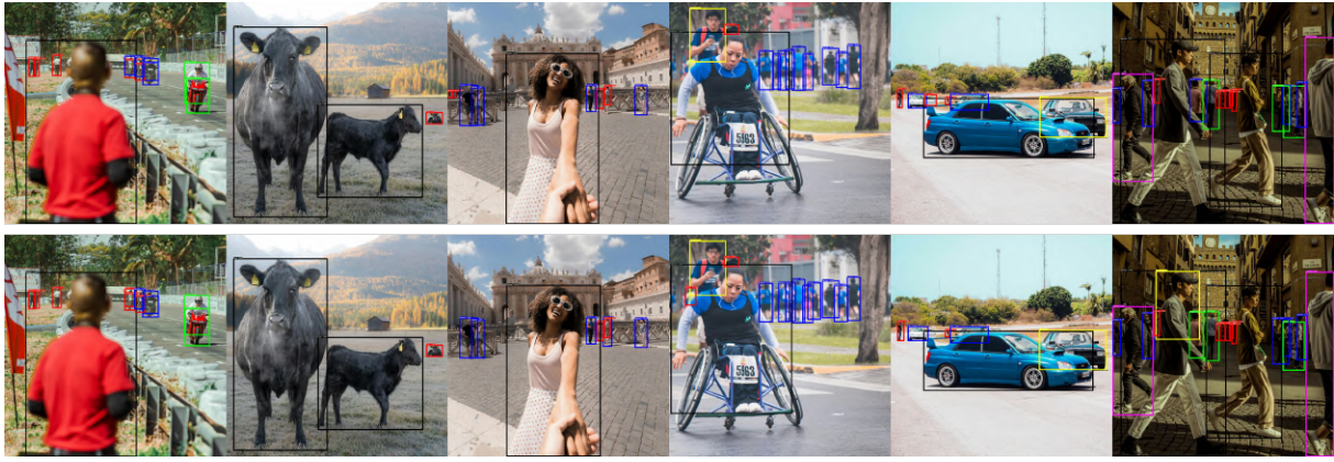
Fig. 6: Six images processed by YOLOv7 and YOLOv7-e6e using the proposed method. The top figure shows the objects detected by YOLOv7, while the bottom figure shows the objects detected by YOLOv7-e6e. The colors of the bounding boxes (BB) in the images are changed according to the sizes of the detected objects: (micro: red, very tiny: blue, tiny: green, small: yellow, medium: pink, large: black).
