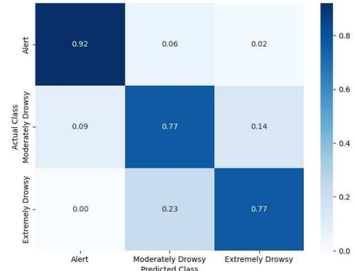
Fig. 5 Confusion Matrix for the Final Model Using Fp1 and Fp2 EEG Channels, HRV Features, and Driving Time
